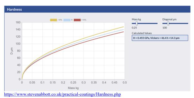
One way to measure hardness is by pushing a Vickers square pyramidal diamond tip into the surface with a known load, F. You measure the diagonal width, D, of the mark you've created and calculate the hardness
