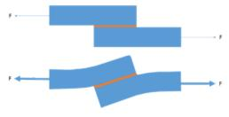
Why are there peel forces in a lap-shear joint?
