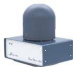
Do the same thing with the particles in NMR tubes and place them not into a fancy NMR spectrometer, but a table-top device (image courtesy of Mageleka) to measure T1/T2 relaxation rates.
