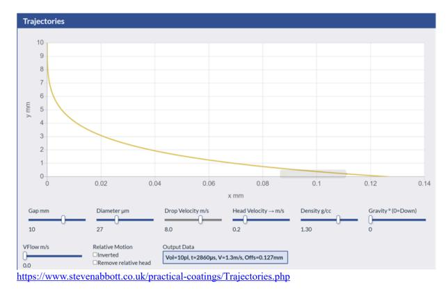
The app answers all 3 questions, but the gravity and deflection issues are not relevant to this book. What is important is that a typical 10pl drop (you define drop diameter and its volume is calculated for you) coming out of the head at 8 m/s lands on the substrate after a 10mm gap at 1.3m/s.
