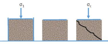
You trap some powder in a box and compress it with stress  $\sigma_1$ . You removed the sides of the box and press till you reach  $\sigma_c$  at which it cracks. You just need to do this for a series of  $\sigma_1$ values, but because you need to pack the box each time people avoid this and use something like a Jenike box
