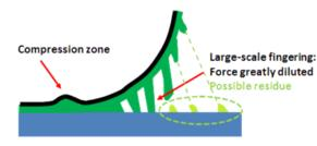
Which brings us to the peel test. This is at last a direct measure of what most of our customers (think they) want. Because adhesion is a property of the system, the peel test is not as simple as it might seem:
