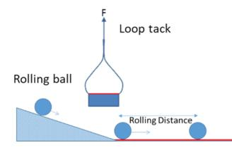
There are two tests that are scientifically valueless yet often used for QC testing: Rolling Ball and Loop Tack Tests. Although simple and convenient, there is a risk that their lack of scientific meaning allows you to miss crucial changes in the PSA properties.
