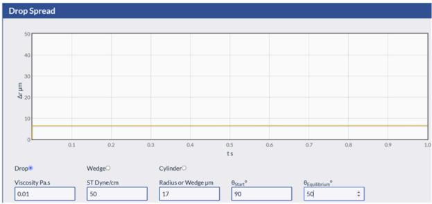
that the drop goes near instantly to 48  $\mu$ m, and stays there pinned at the 50° limit. Inkjet printing is one of the rare portions of formulation science where contact angle is of crucial importance.
