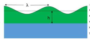
A coating will often contain some sort of line defect visible during creation (coating head, brush, roller) but invisible once dry. As the wet coatweight is reduced the same wet defect now shows up in the dry coating. Why? Because the defect has not had time to level out. The reasons for this are not obvious until Orchard levelling theory is invoked.
