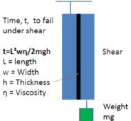
For example, the classic PSA shear test shown in the diagram is only a test for passing the shear test. It has very little relationship with the shear properties of the PSA for a good reason – it often fails in peel, a fact common in shear testing. So the formula shown in the image is not applicable, much to the puzzlement of people who think that the shear test provides information about shear behaviour.
