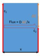
If we are concerned with fragrance/flavour molecules escaping, so-called flavour scalping, then we can assume that the external concentration is zero and that we have a packaging film from a single ingredient (we will modify this later) of thickness x.
