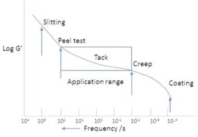
Although your PSA may be designed for a modest temperature range, it will experience various timescales in use. If it is perfect when tested slowly yet fails at high speed, then that might make it useless for a specific application. Here are some typical timescales and an indication of how G' changes over those timescales. We shall shortly see what those G' numbers are, but you already know from Dahlquist that the Tack G' at  $10^{0}$ /s (i.e. 1/s) must be ~0.1 MPa.
