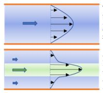
There are two problems with trying to clean out a pipe full of one fluid by pumping another fluid through it. The first, this time showing <u>Flow\_Poiseuille Flow</u> is that the velocity of the fluid at the surface is still zero:
