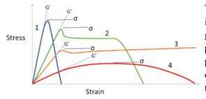
To understand the behaviour at high strains, the ideal test is on a tensile tester. This is relatively unpopular, but gives the most direct information. More popular is the probe tack test which has a tricky relationship to PSA performance (described below) but is quick and convenient. In either case you get curves something like this:
