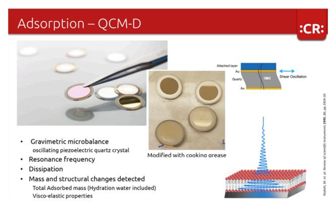
Put a quartz crystal into your solution and get it to oscillate at its resonant frequency. Because of the viscosity of the liquid, this frequency will be different from that in air. If you have a QCM-D machine (D for Dispersion) you can see how the amplitude of the oscillations decay when the stimulating signal is switched off.
