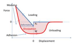
The more productive idea of "adhesibility" is described in an app, <u>https://www.stevenabbott.co.uk/practical-adhesion/</u> adhesibility.php, that invokes a nanoindenter or JKR-style machine for measuring the hysteresis effects that illustrate the potential for adhesion. The initial jump in the loading curve gives the pure surface energy, and the subsequent cycle during loading and unloading gives you a lot of information about modulus and the dissipation that is a key part of adhesion.
