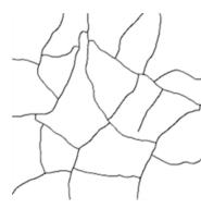
If the drying process happens too quickly, before the sintering takes place, then the paint can start to show mud crack patterns, such as the one shown here, taken from the app, <u>https://www.stevenabbott.co.uk/practical-coatings/</u> <u>Cracks.php</u>, which describes the phenomenology while giving little advice about how to solve the cracking issue. It's interesting that the cracks join at right angles, though sometimes you get patterns that crack at 120°. Interesting, but not so helpful.
