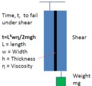
The classic, official PSA shear test shown in the diagram is only a test for passing the shear test. It has very little relationship with the shear properties of the PSA for a good reason – it often fails in peel, as we saw with the lap joint. So the formula shown in the image is not applicable, much to the puzzlement of people who think that the shear test provides information about shear behaviour.
