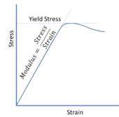
You clamp a sample into the jaws of an Instron-like machine and apply a *stress* (force per unit area) and measure the strain (% change in length). For a while the stress is proportional to strain and the gradient, Stress/Strain is the modulus. Stress is in Pa, strain is unitless, so modulus is in Pa, more usually MPa or GPa.
