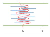
Everyone loves the idea of taking a cheap, natural clay and creating a tortuous barrier layer. For a thickness L, a molecule has to travel a distance  $L_B$  to cross the barrier. The more clay we can pack in, the more tortuous the path and the better the barrier. The problem is that clays, when well-dispersed, add considerable viscosity to the dispersion so there is always a trade-off between the amount you would *like* to add and the amount you *can* add.
