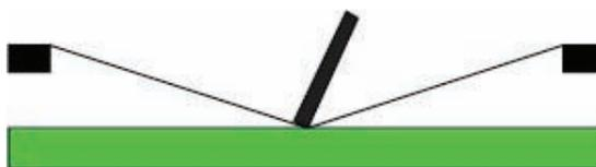
*Middle of the mesh, relatively low pressure required, medium distortion*
