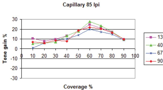
Effect of exposure time on tone gain for an 85lpi test positive in a capillary stencil. There is very little change from increased exposure times because there is very little scattering from the smooth stencil surface.
