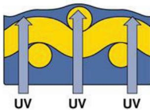
EFFECTS: All the emulsion is fully hardened and the stencil will provide the optimum resistance and durability.
