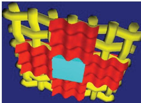
However, a typical low-Rz stencil is high EOM and a high EOM gives you a bigger ink deposit which also spreads (slumps) more to give you dot gain.
