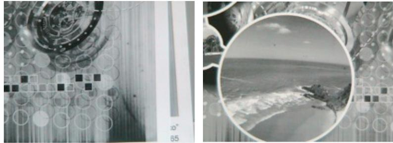
*Under magnification it can be seen that the ink is severely undercutting the stencil.*
