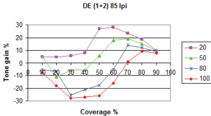
The same experiment using a 1+2 Direct Emulsion (high Rz). With increased exposure time, the scatter from the Rz caused dramatic filling-in of the dots, i.e. severe undercutting.
