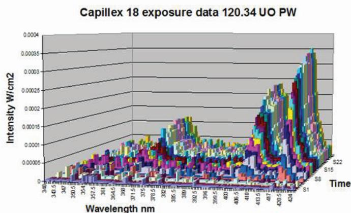
As exposure time increases more of the light emitted by the lamp passes through the stencil as less is used in the crosslinking reaction. If only 418nm light is considered then the reaction can be seen to be complete when the light reaches its maximum:
