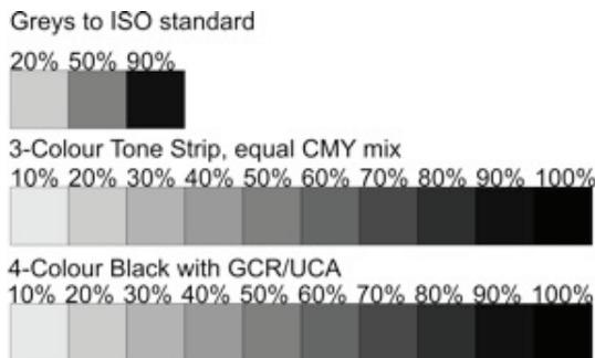
*A simple test strip that would let you measure the CFI of any set of print sequences.*
