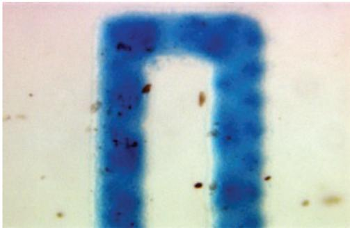
*The mesh marking is the dots of darker blue*
