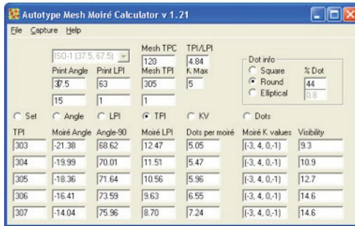
Figure 5 The moiré does not change all that much (e.g. the angle changes from  $-21.38$  to  $-14.04^\circ$ ) when the thread count changes by a modest amount.
