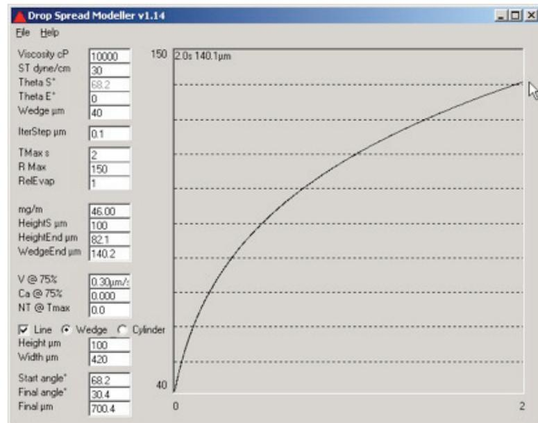
*The Drop Spread software models the 100 $\mu$ m high, 500 $\mu$ m wide line*
