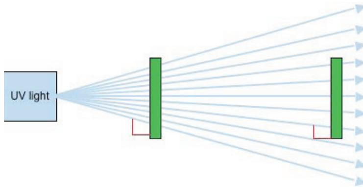
As the distance between the light source and the vacuum frame increases so less light hits the stencil. This means that the time to achieve full exposure will increase. The formula for calculating this is:
