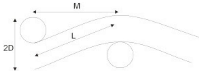
The total height of this ideal mesh is twice the mesh diameter,  $2D$  and the spacing  $M$  is  $1/TPM$  (Threads Per Micron)
