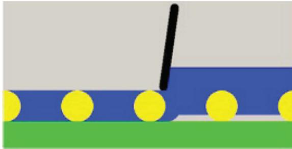
*In control: the squeegee filling the mesh and scraping off the excess ink*
