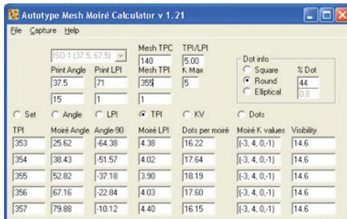
Figure 6 The moiré now changes by a large amount (e.g. the angle changes from  $25.62$  to  $79.88^\circ$ ) for the same small change in mesh count.
