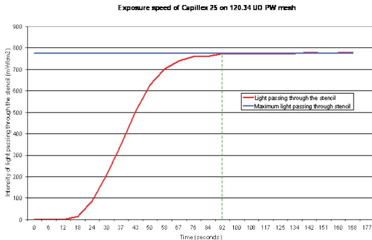
*In this example the light reaches a maximum at 92 seconds and so this is full exposure.*
