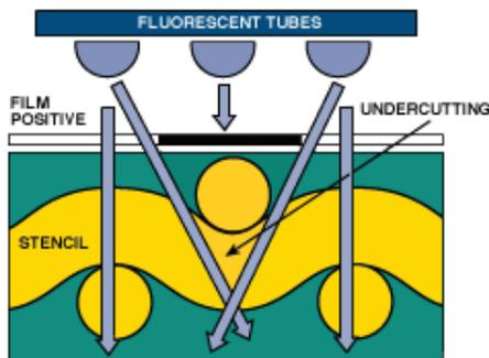
From a practical point of view poor light geometry effects do not present a problem when processing general work, i.e. lettering down to about 6 point and halftones of 65 lines (25 cm) or coarser.
