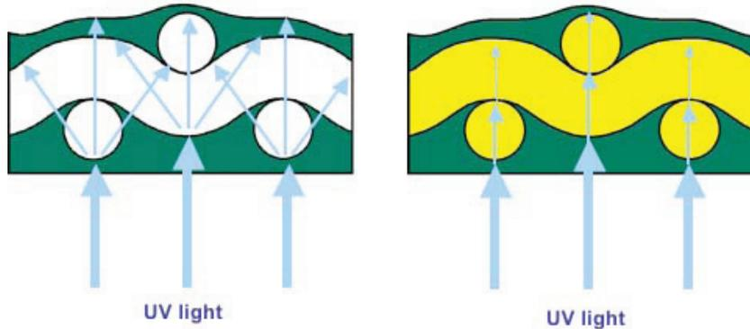
White mesh transmits and scatters light, yellow and orange mesh absorb the wavelengths needed for the crosslinking reaction, but scatter far less of the light.
