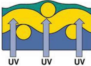
EFFECTS: Emulsion appears slightly soft on squeegee side. Stencil will scum if not washed out properly. Durability is compromised. Stencil is harder to de-coat.
