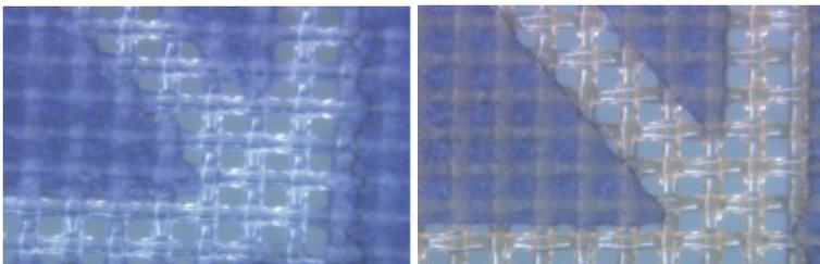
4. Stepping caused by image angle to the mesh
