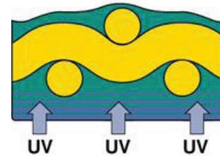
EFFECTS: During washout the image would appear and the stencil would probably start to come away during washout.
