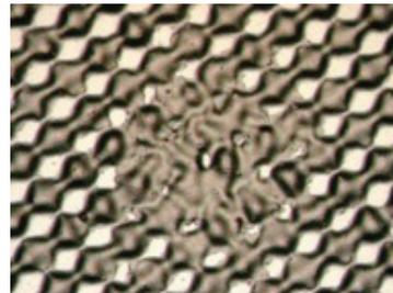
*There is still evidence of the intended image within the blemish which means that it is not a pin hole in the stencil.*
