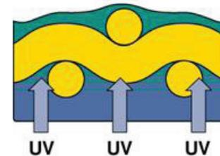
EFFECTS: The stencil would probably be damaged by a strong washout spray. The emulsion appears soft on the squeegee side.
