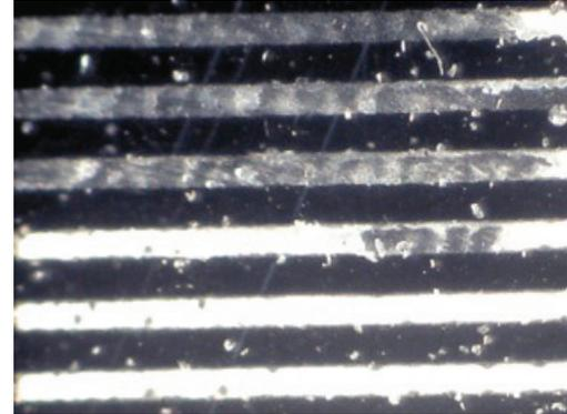
We deliberately waited some time after the flood stroke before printing – and used an ink with no added retarder. Naturally the ink had dried in, blocking some of the holes, giving the classic drying in pattern. We could also achieve drying in only at the image at the start of the print stroke. This is because the ink remaining in the mesh after the print had longer to dry in before it was re-flooded.
