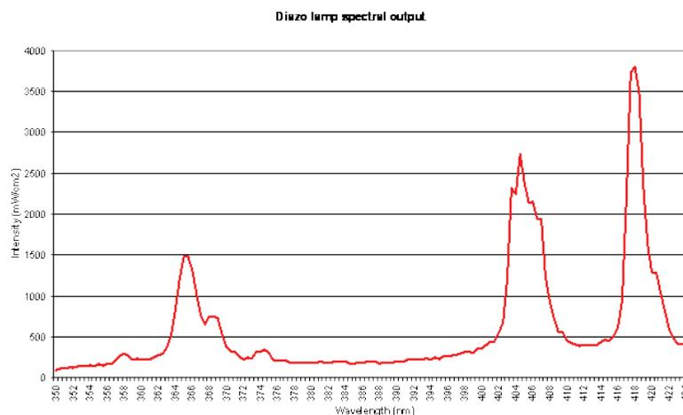
If the spectral output of the lamp and the adsorption of the sensitizer match, then the light energy will be used by the sensitizer for reaction. Once the reaction is complete then light which is not absorbed by the pigments in the emulsion and dye of the mesh will pass through the stencil. This light can be detected and measured with a radiometer and then plotted as illustrated:
