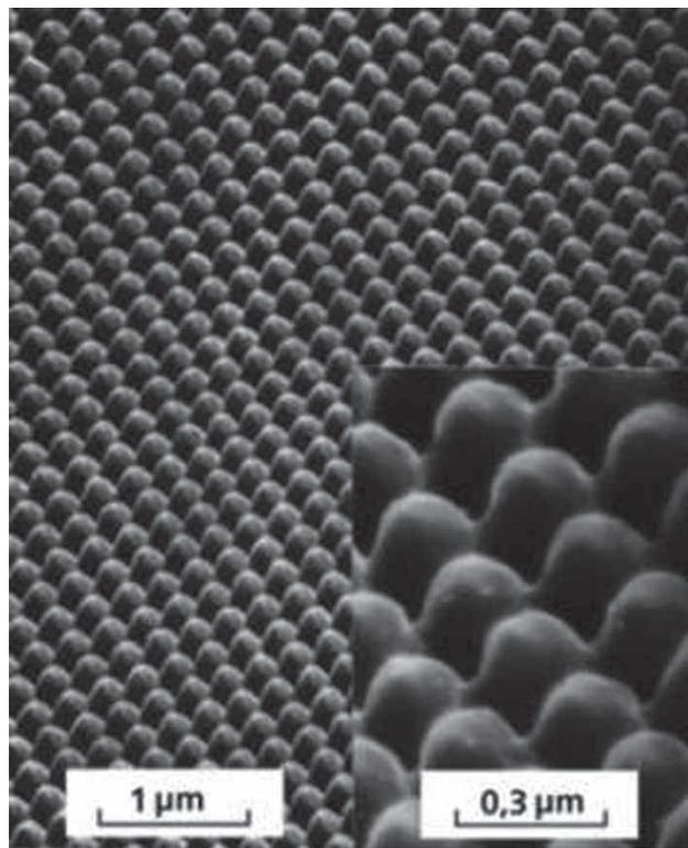
**Fig. 1** Motheye structure replicated into a hardcoat polymer surface by MacDermid Autotype. (Image courtesy of Fraunhofer ISE)
